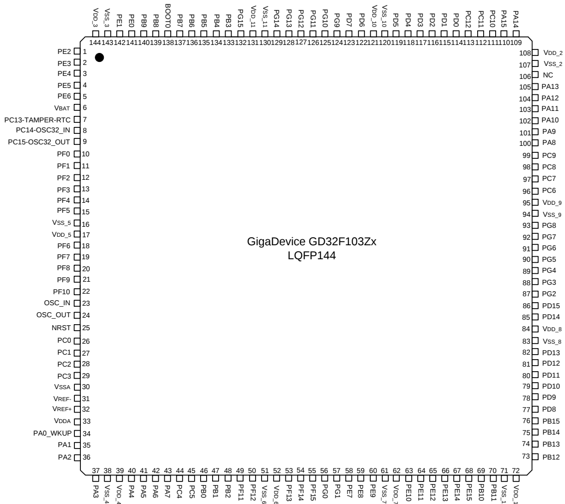
Figure 3. GD32F103Zx LQFP144 pinouts
